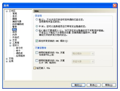
In the pop-up dialog box, select VBA, on the right do not check the "delay load VBA", then OK, and exit the application CorelDraw.
