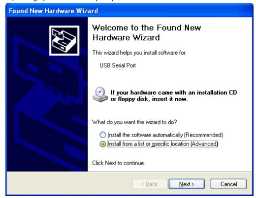
Select "Install from a list or specific location [Advanced]" and then select "Next". The remaining operation is consistent with the foregoing. Until the following dialog box appears.
