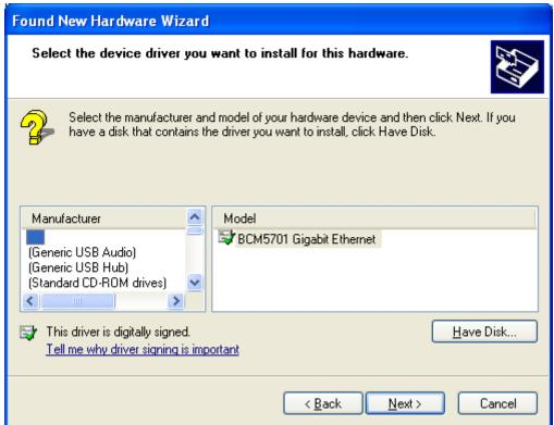
Select "Have Disk", and manually navigate to the driver to the driver location, select the file ftdiport.inf.
