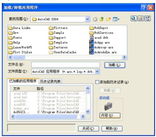
Select "Add" button in the pop-up dialog box. In the AutoCad directory, manually locate and select acad.dvb,acad.lsp. And loading these two files.
