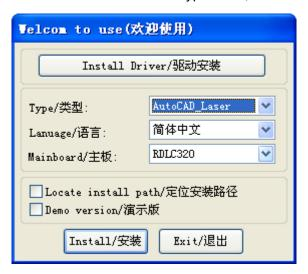
Setup will automatically install the RDCAM plug-in software to all versions of AutoCad that were installed on the operating system and pop-up dialog box.
