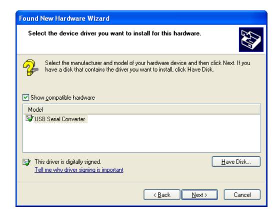
After the installation process, within the Device Manger will show "USB Serial Port".
